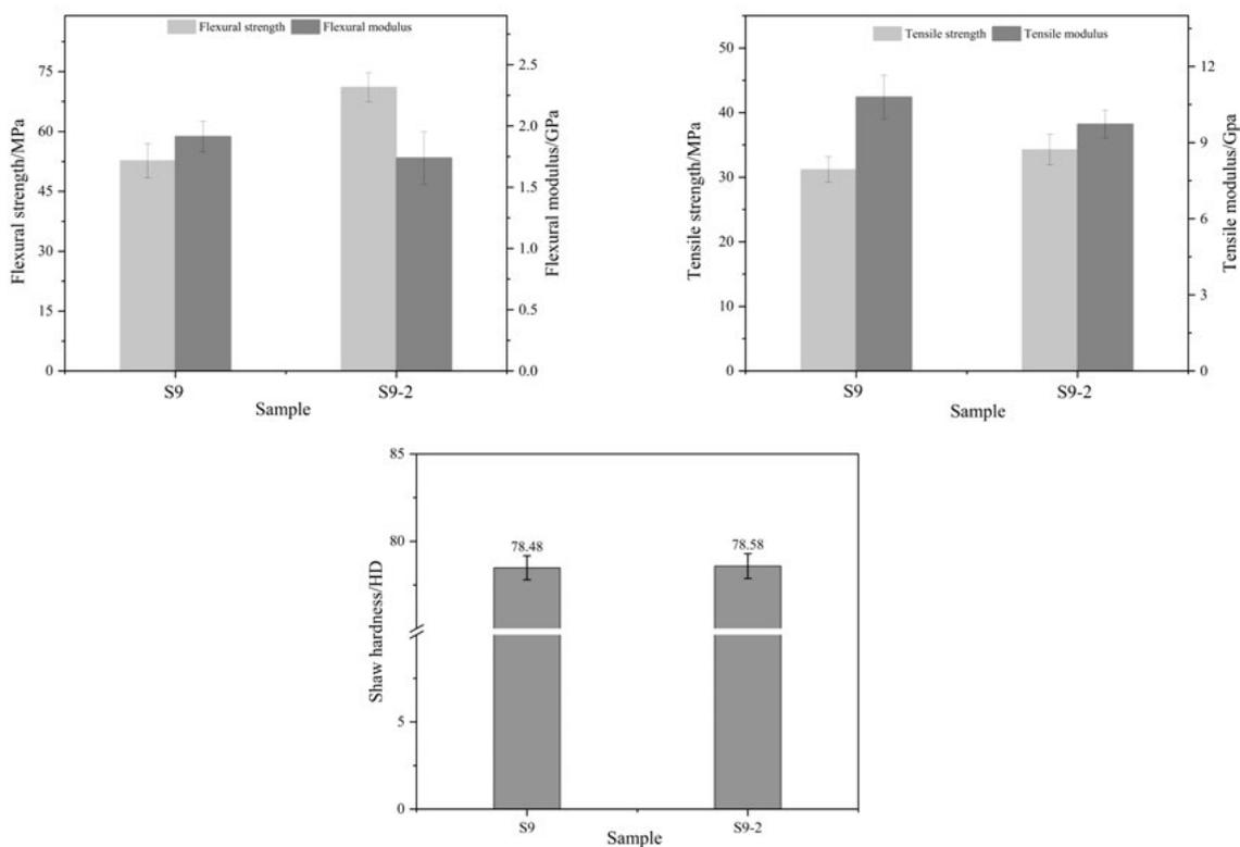
Figure 8 Effect of modification treatment on mechanical properties of composites
