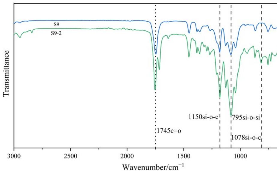
Figure 7 FTIR spectra of biochar modified composites
