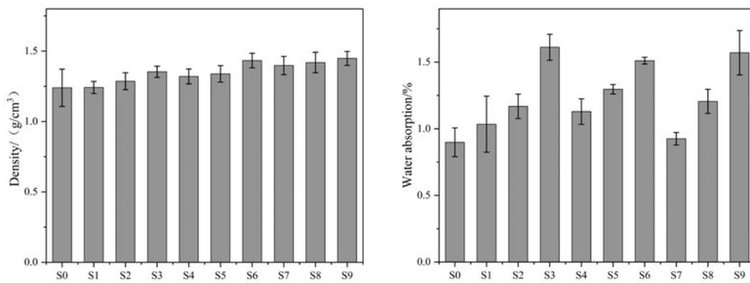
Figure 4 Density and water absorption of composite materials
